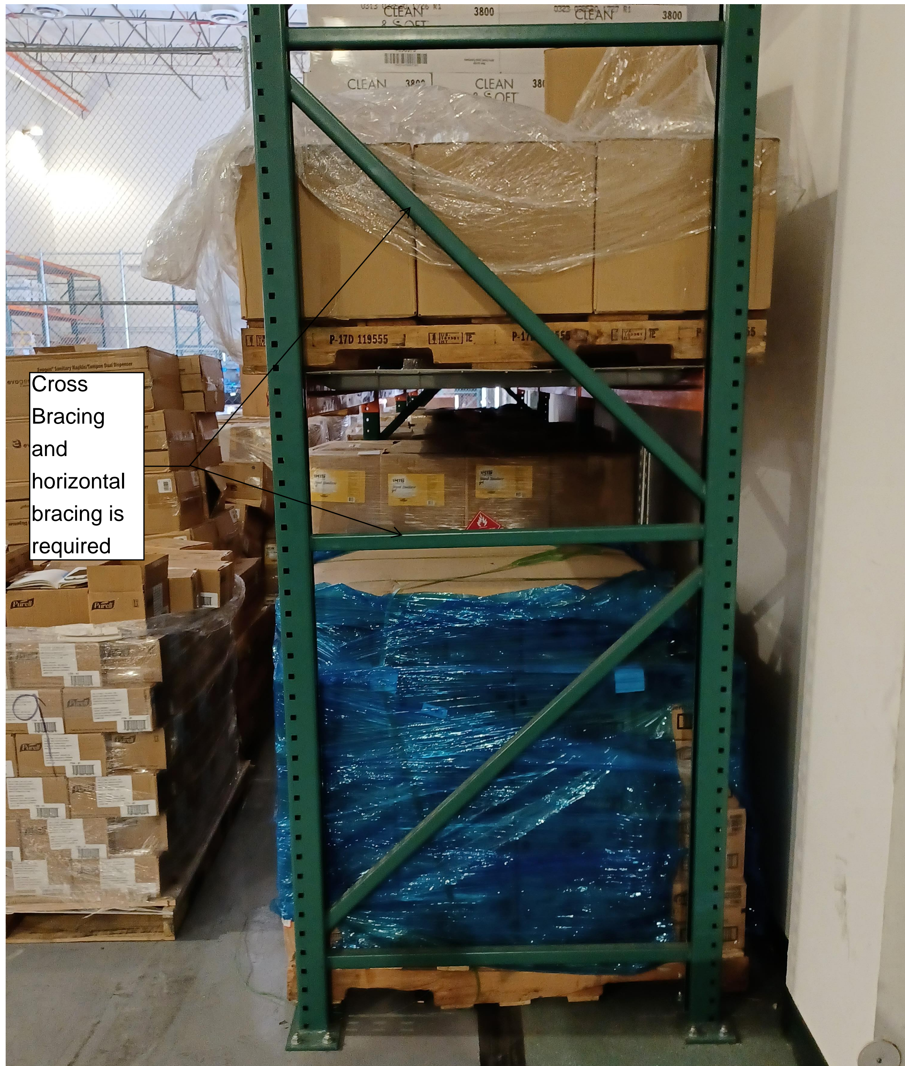
1 Upright bracing configuration
